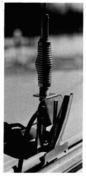
Construction of the 2-meter, quarter-wavelength, mobile whip antenna. Parts were scrounged from CB supply stores and the author's junk box. The antenna is easy to unclip and remove when you leave your car unattended.
